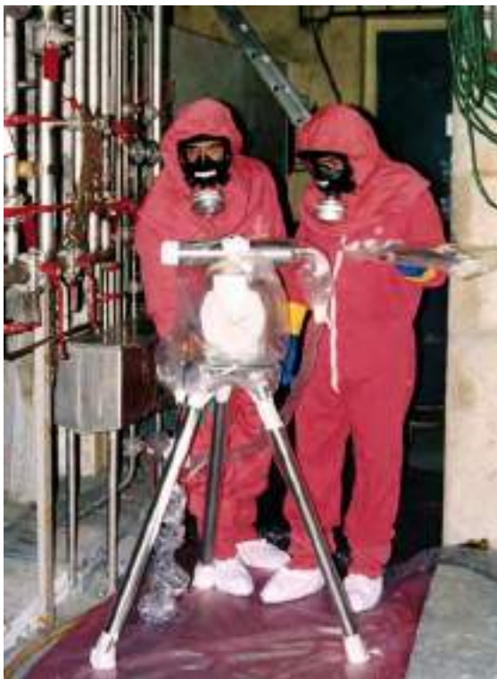
In situ radiological inventory prior to decontamination with Cartogam detection head mounted on Pan and Tilt and tripod.
