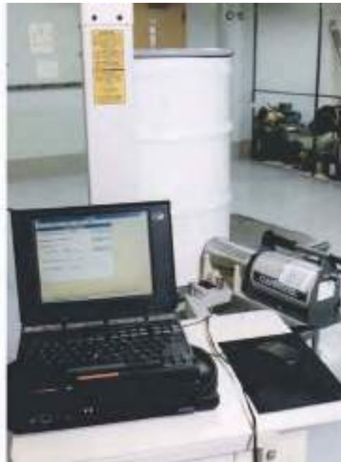
Fig. X-6. A mobile FRAM system measuring the isotopic composition of the contents of a 200-liter waste drum.
