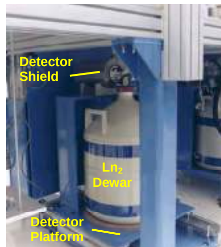
Fig. XIV-4. A closeup of the FRAM isotopic analysis station in the ARIES NDA system.
