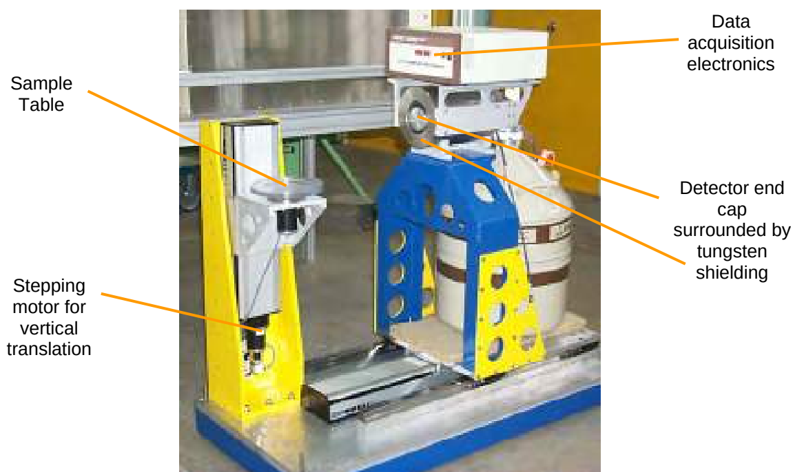
Fig. XIV-1. The hardware for the IIU at the Los Alamos Plutonium Facility is shown before its installation.
