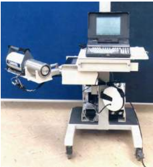
Fig. X-5. A mobile PC/FRAM system configured on a commercial thyroid scanner cart for use at the Los Alamos Plutonium Facility. The shielding around the detector is 0.75 in. of machinable tungsten.
