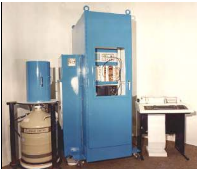
Fig. III-2. The LAPIS plutonium isotopic analysis system implemented at the Savannah River Plant.
