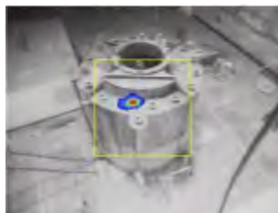
Figure 3 Gamma Image #4 obtained for the High Rad Tank on cell 35
