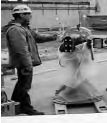
Figure 3. Plastic wrapping of RadScan 600.
