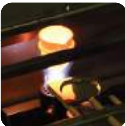
■ Heat crucible in melting furnace
