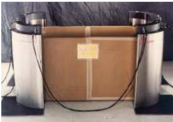
The WM3500 can be used with larger objects by separating the pillars.
