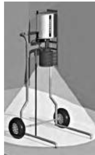
7b: Shield and collimator installed.
