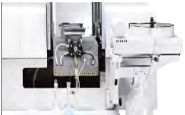
Figure 5. The AS-800 furnace autosampler easily swings into place.
