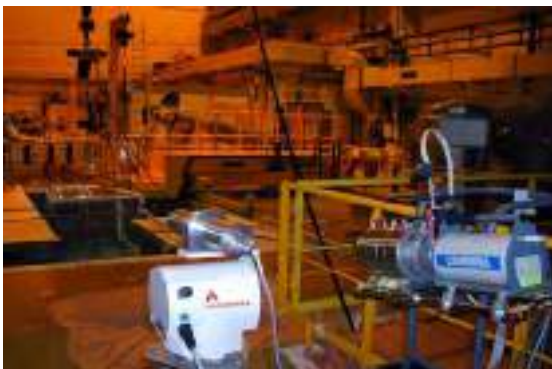
Cartogam in association with ISOCS and Mercurad for easy localization and activity measurements of hot spots.
