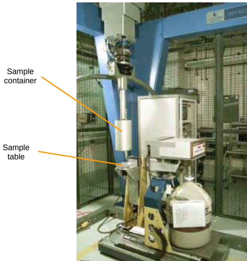
Fig. XIV-2. The ROBOCAL robot is about to place a container on the sample table of the IIU at the Los Alamos Plutonium Facility.
