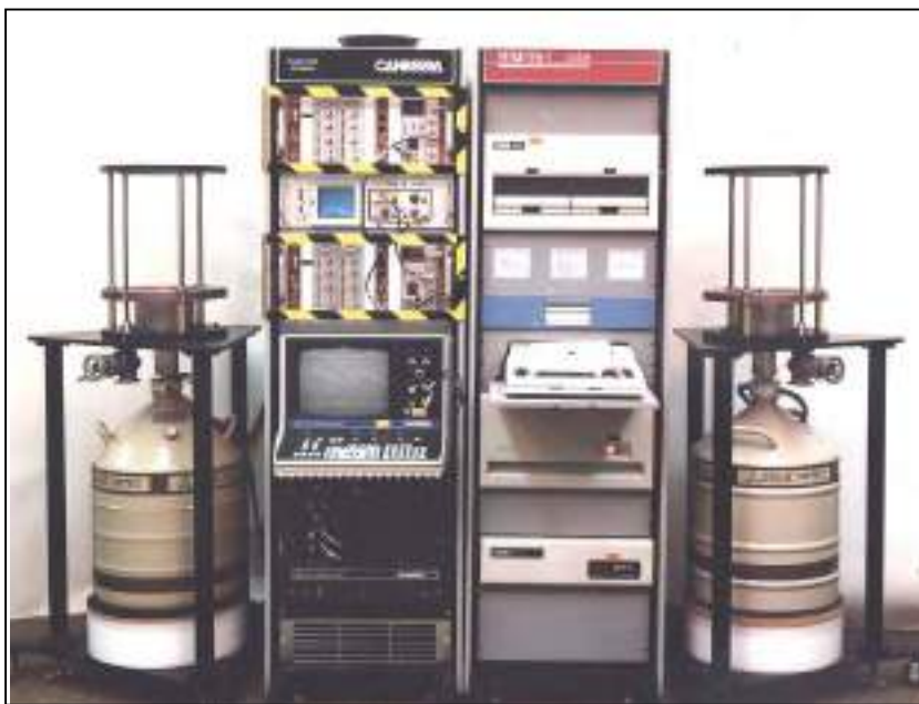
Fig. III-1. The MUDPI plutonium isotopic analysis system implemented at the Los Alamos TA-55 Plutonium Facility in the early 1980s.
