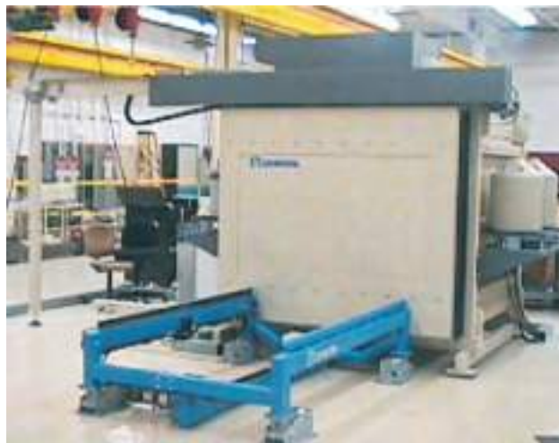
Figure 1. Waste Crate Assay System (WCAS).
