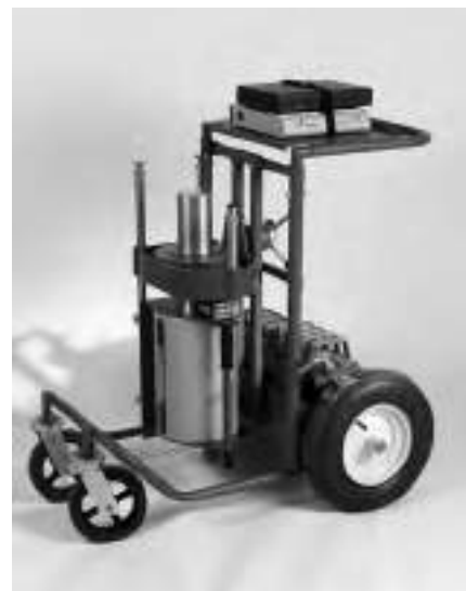
Figure 10 ISOCS shield ready to move to new location; all shield accessories fit into carrying tray on back; computer and MCA can be strapped down to tray on top.
