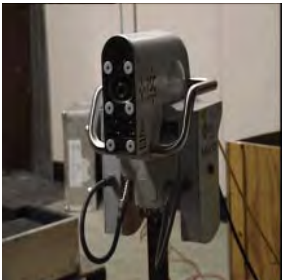
Figure 1. RadScan 600 inspection head.
