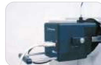
Pulsed Dynamic Focusing MALDI (PDF-MALDI) Source
