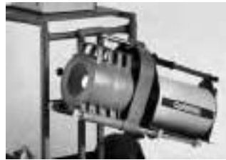
5b: The same detector with the 50 mm Shield and a 90° Collimator installed.
