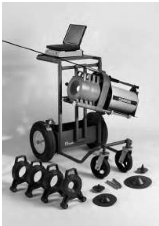
Figure 1 The ISOCS Shield Systems and all of their available components installed on an RDC Ge Detector with a Big MAC Dewar. (See Figure 3 for more details.)
