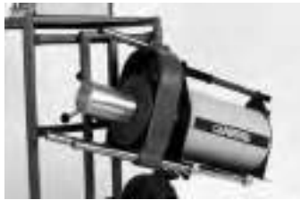
5a: The detector and mounting assembly. Note that the detector has the RDC chamber and that the backshield is installed.
