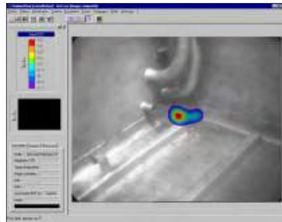
Cartogam – superimposition of visible and gamma images without parallax. Gamma hot spots are quantized using a color scale.
