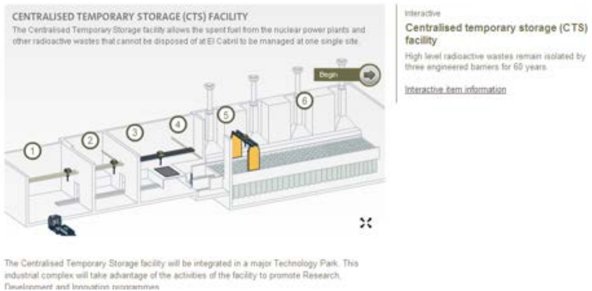
Fig. 33 – Centralised Temporary Storage facility scheme
