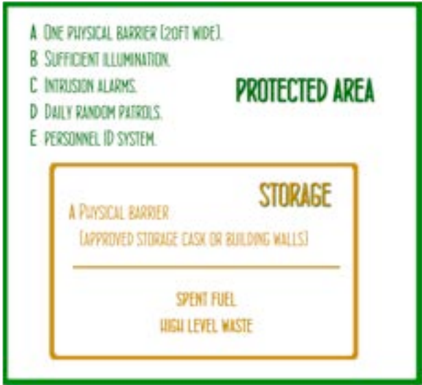
Fig. 6.5: Physical Protection System at storages in USA.
