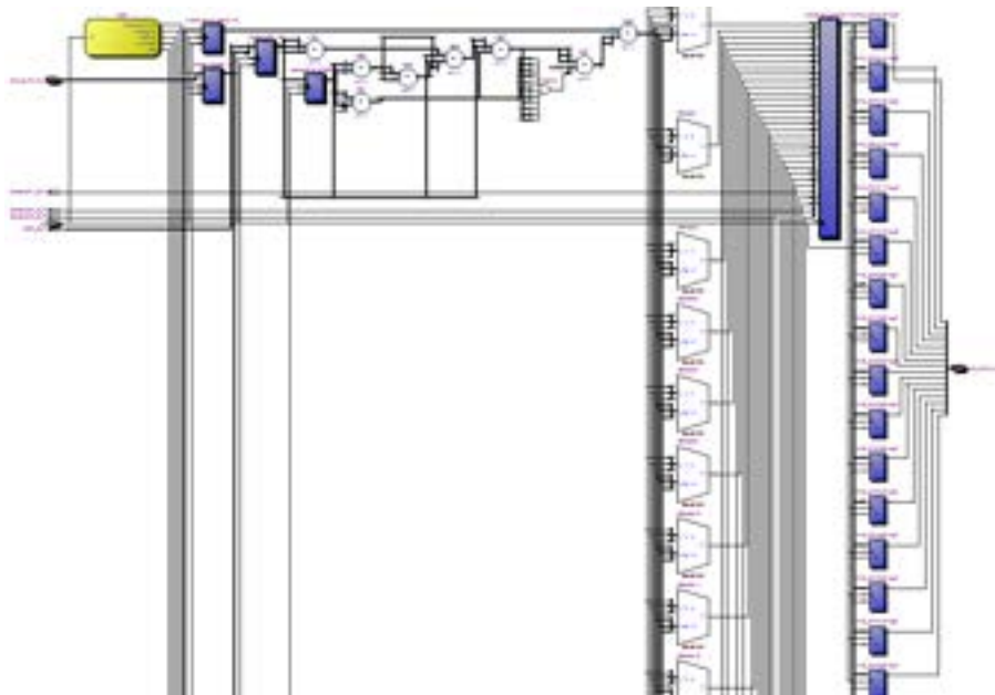
Figure 46: Register Transfer Level of main PID digital core implementation in FPGA
