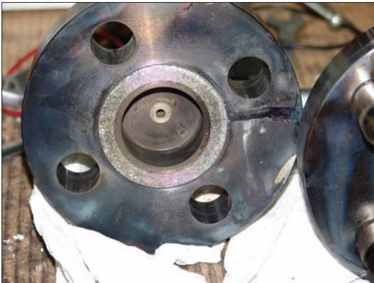
Fig.5. 7 – Phlogopite mica gasket after testing
