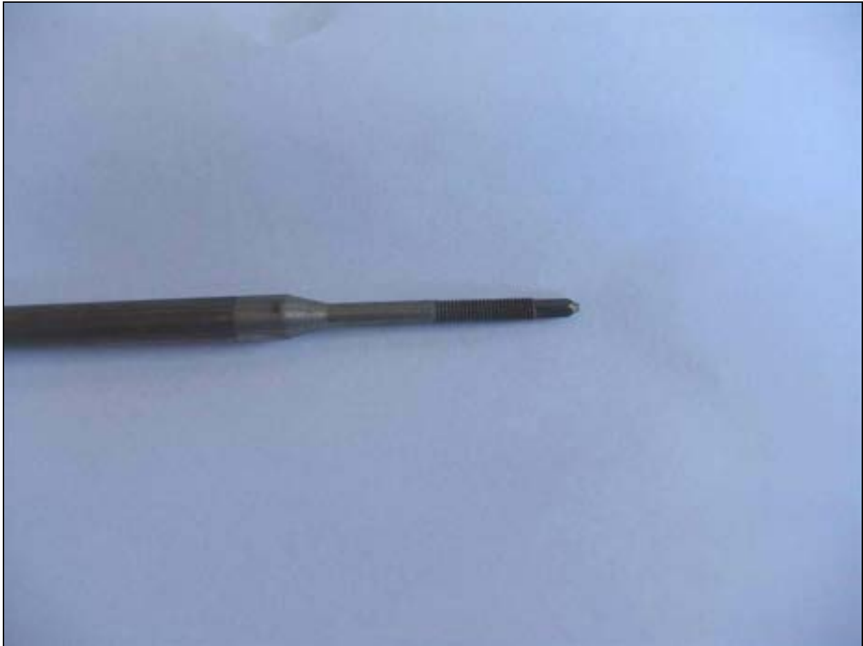
Fig.5. 2 – SPES-2 heater rod upper termination
