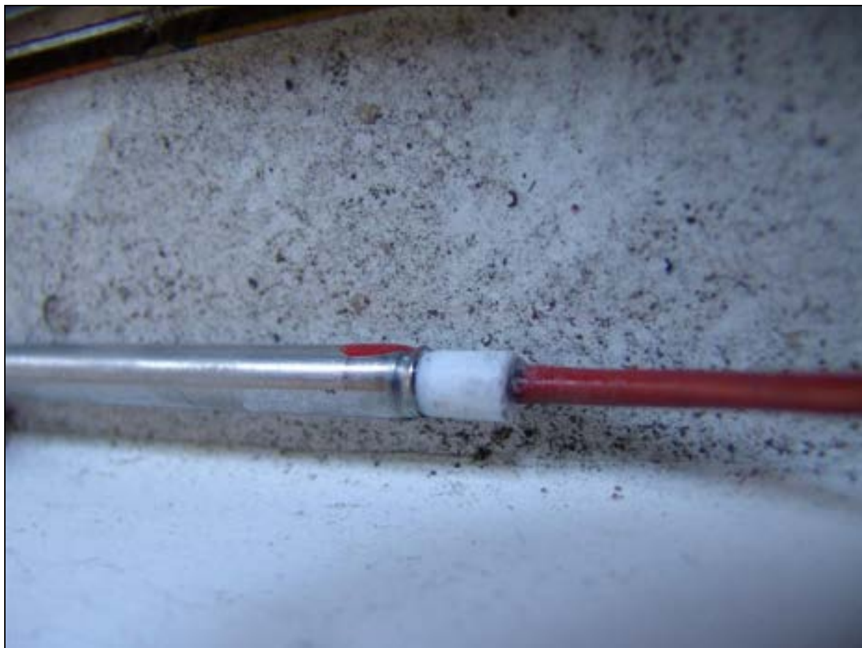
Fig.5. 1 – SPES-2 heater rod lower termination
