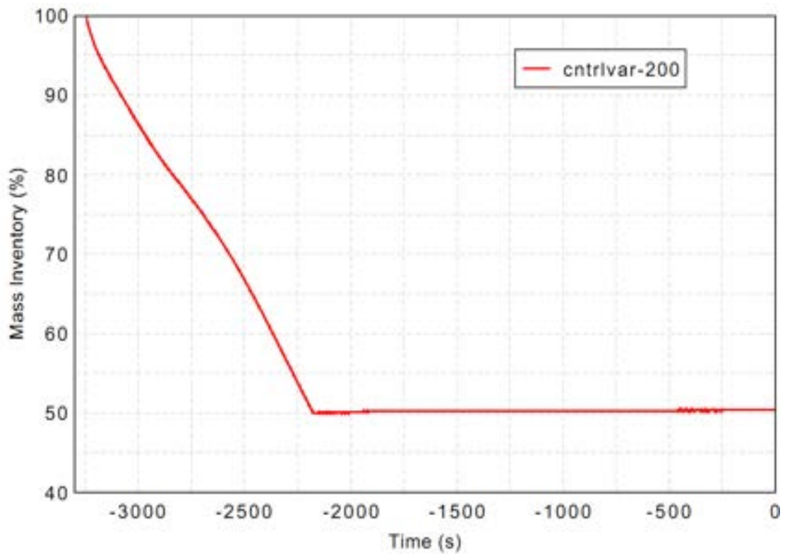
Figure 13. Conditioning phase: Primary side mass inventory
