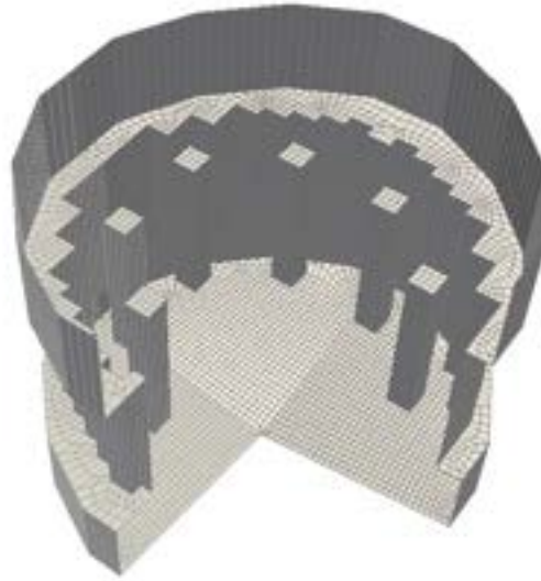
Figure 4.3: Core, lower and upper plenum reactor coarse boundary mesh
