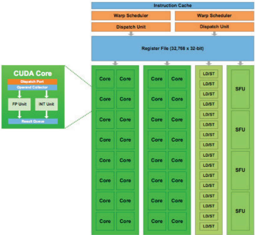
Figure 3.53: Streaming multiprocessor (SM) GPU structure
