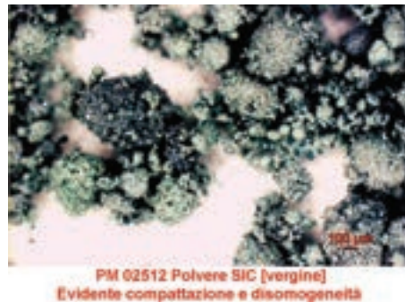
Fig. 77 – Si-C powder - 20°C.
