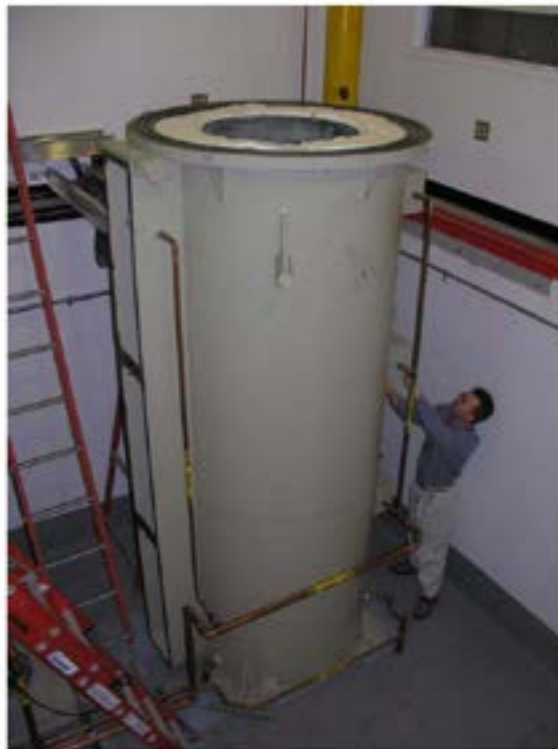
Figure 7. Production-scale CWF furnace.
