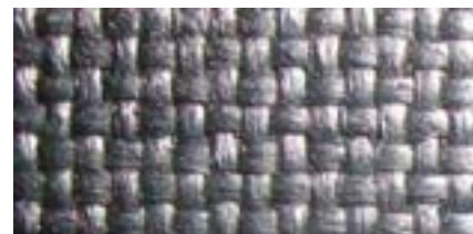
2D Textile Architecture (SiC/SiC)
