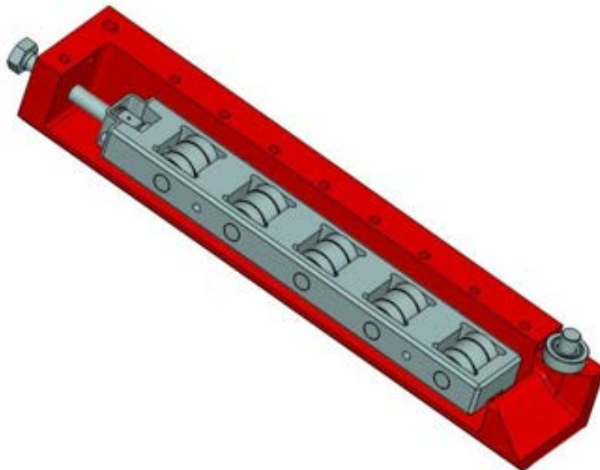
Figure 10 – Skate frame with bearings (gray) inserted in the L-shape structure
