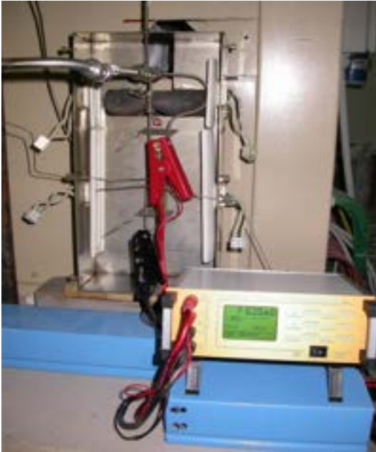
Figure 11: general view of the measurement apparatus, with the nano ohm meter close-up
