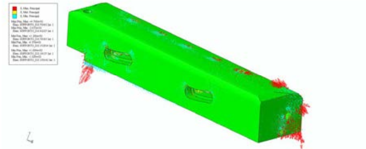
Fig. 25 - Direction of the principal stresses (outside view)
