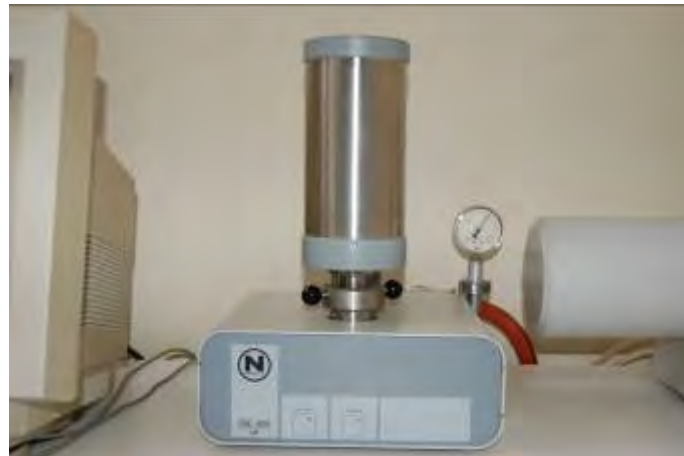
Fig 2.9: Differential thermal analyser apparatus
