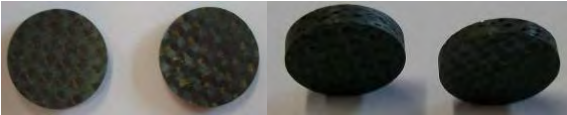
Specimens for the thermal diffusivity measurement
