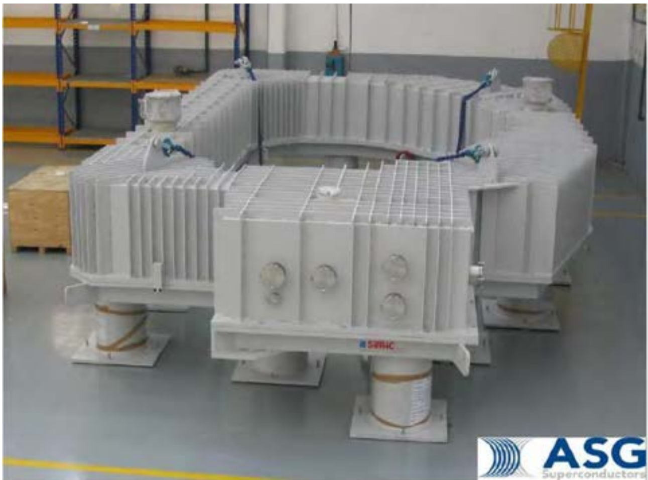
Figure 9 Vacuum chamber to perform final test on coil.
