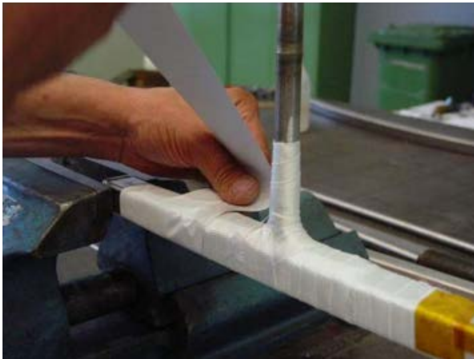
Figure 13 He inlet insert covered by glass tape to perform the insulation and the related electrical tests.
