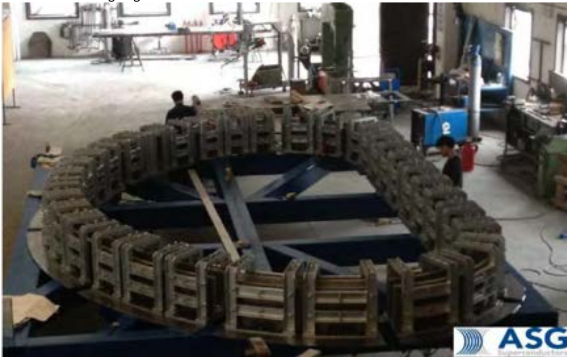
Figure 6 Impregnation mould during final tests before installation in Genoa.
