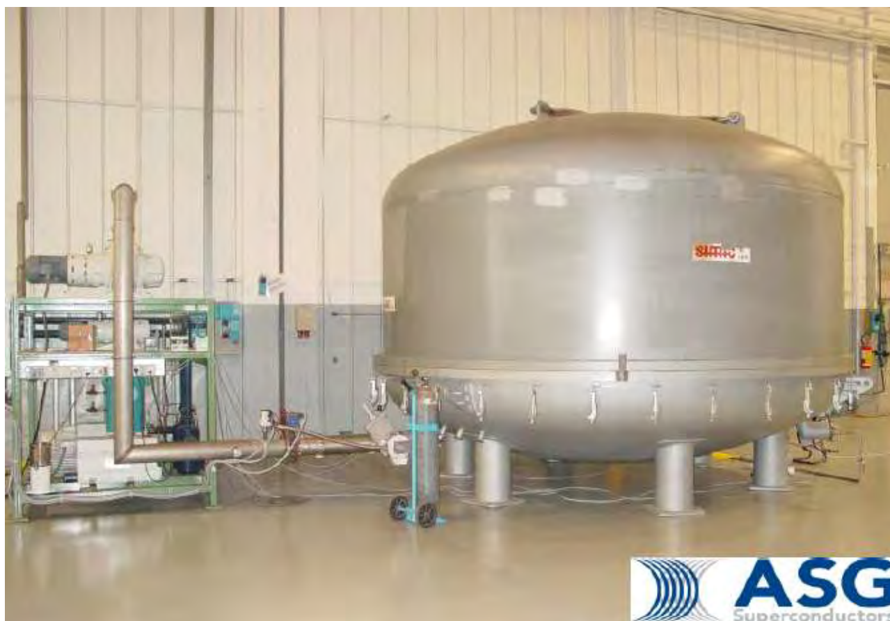
Figure 1 Vacuum chamber and pumping system for acceptance tests on spooled conductors.
