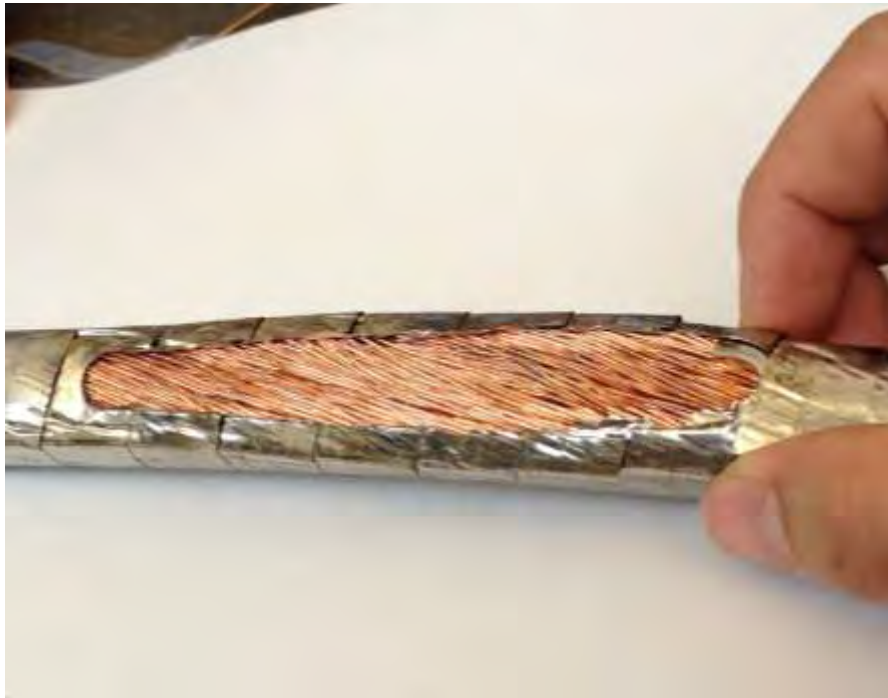
Figure 12 NbTi and copper strands underlying the He inlet insert after the destructive examination of the sample to perform measurements of the strand degradation.
