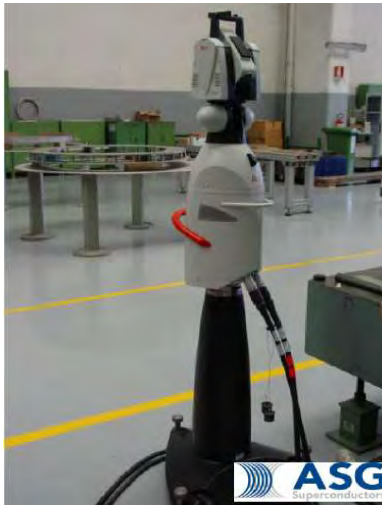
Figure 8 Laser tracker for dimensional survey.
