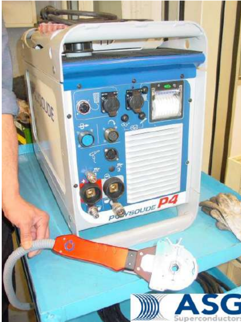
Figure 7 Orbital welding machine for He piping welding.
