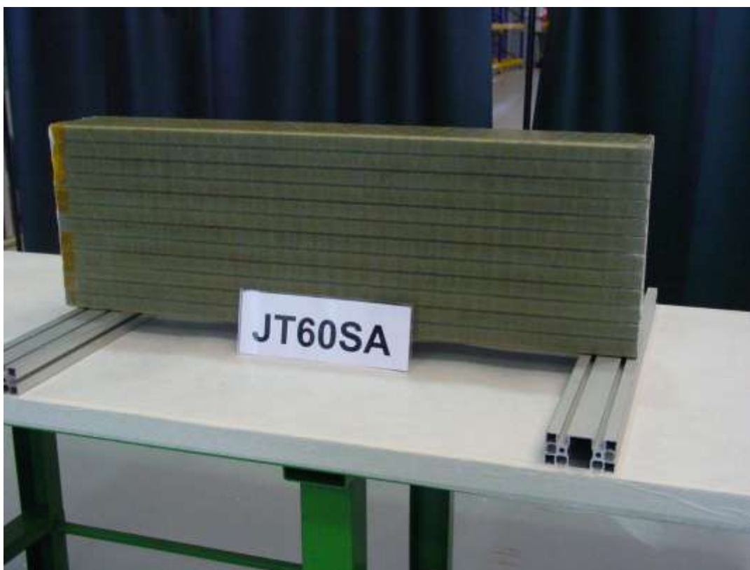
Figure 11 Impregnation beam before the application of the conductive painting and the execution of the associated electrical tests.
