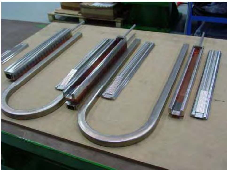
Figure 14. Terminations and inner joint sample preparation.
