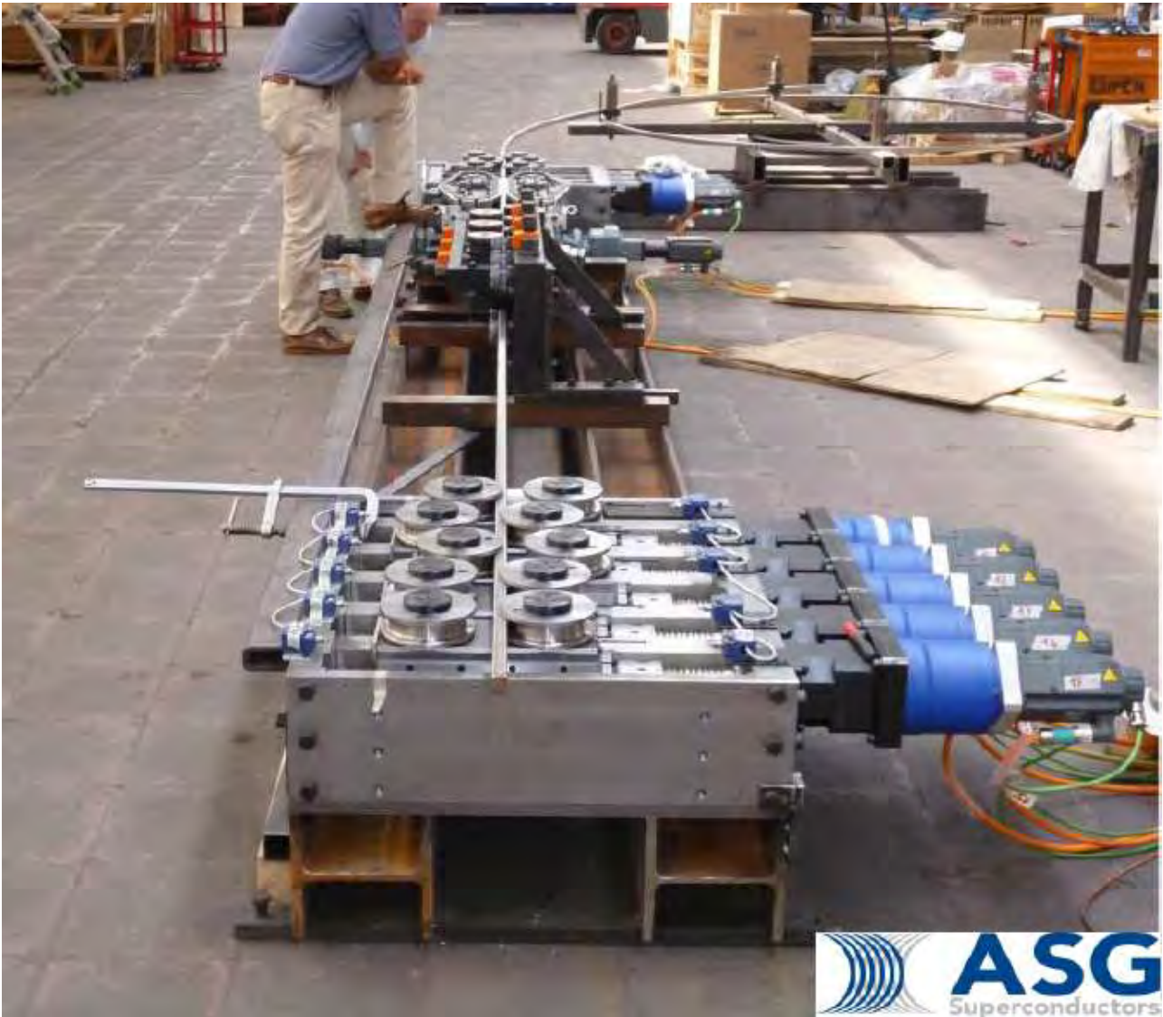
Figure 2 Straightening and bending tools of the winding line during final test before installation in ASG premises.
