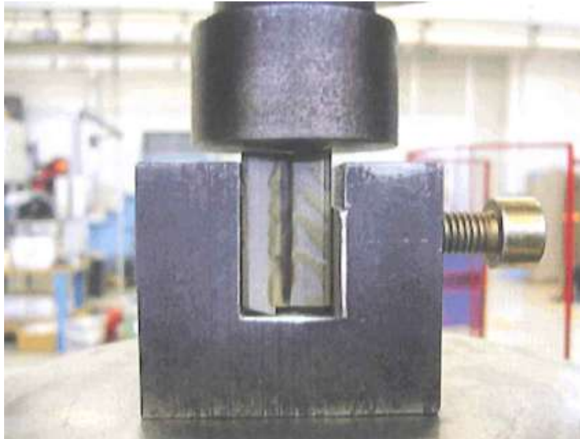
Figure 10 Shear stress sample during the static load at the test facility.
