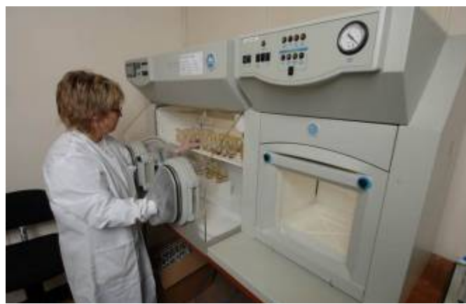
Anaerobic chamber in the Geomicrobiology Laboratory
