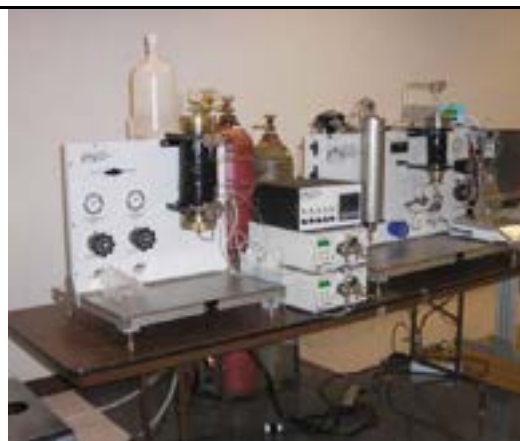
View of the two equipments within the CCSLAB: The MSCL-S system for laboratory core logging & Benchtop liquid permeability system to be upgraded for CO 2 (sc) studies
