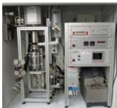
Magnetic suspension balance equipped with steam generation and multiple gas inlet systems.
