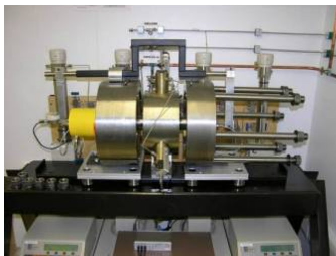
Intrinsic permeability measurement in the TPRL
