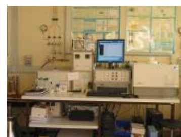
Figure 3 Two NMR devices: 23.7 MHz (left) and 2.2 MHz (right)
