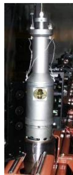
Fig. 4: Fluid cell for IFT-measurements (working conditions: 700 bars and 180 °C)
