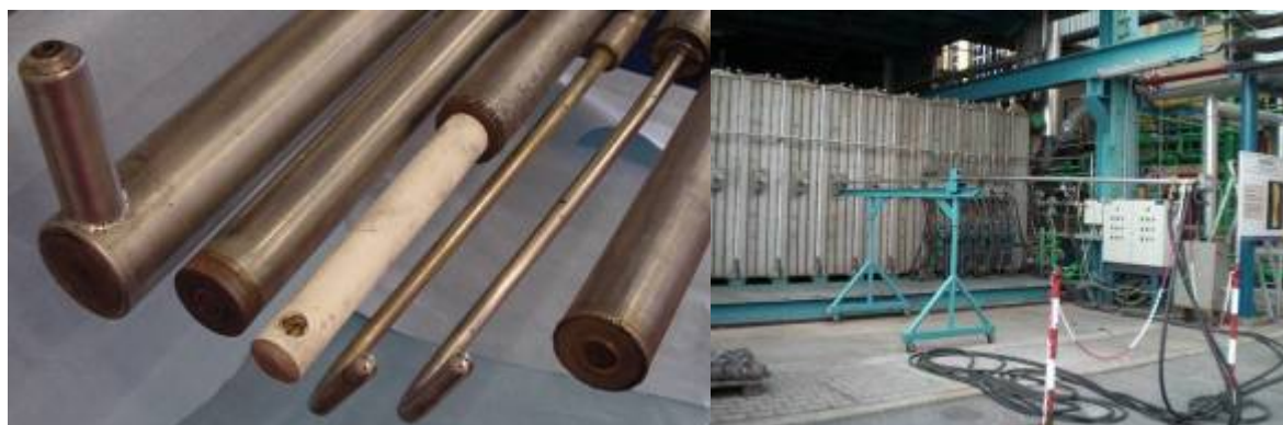
IFRF probes for in-flame measurements in FO.SPER
