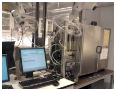
Figure 2. Pictures of membrane gas permeation test rig for single/mixed gas(left), membrane permeation test rig for humidified conditions(middle) and membrane permeation test rig for mixed gas at high pressures (right)
