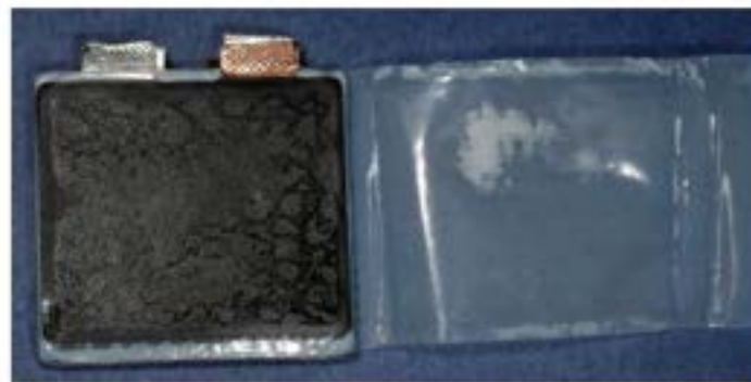
Figure 4 Example of a stacked prismatic cell design
