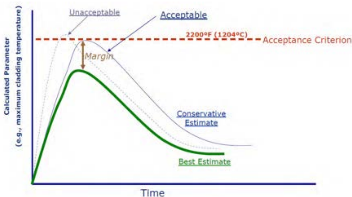
Figure 6- Example of peak cladding temperature acceptance criteria based on deterministic evaluation [30]
