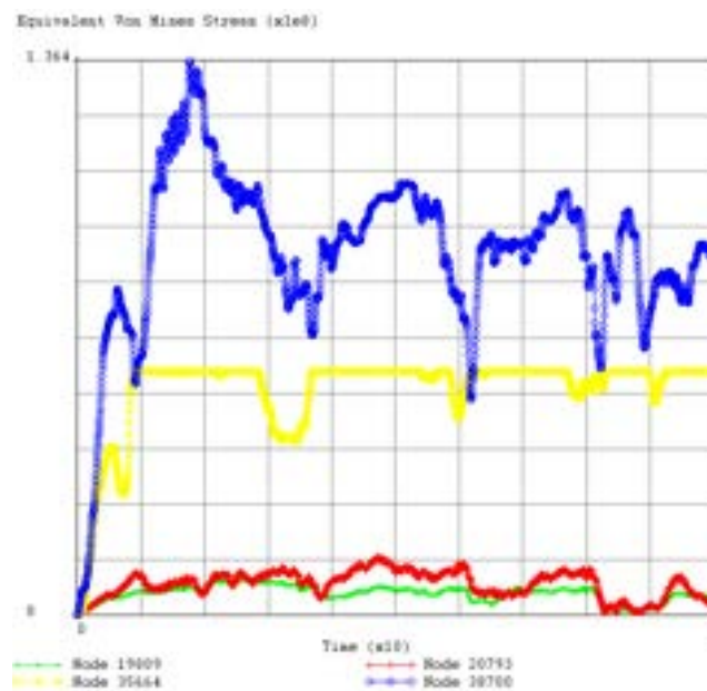
Figure 13. Von Mises stress at several location in the containment structure.
