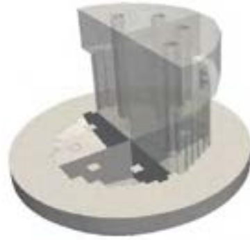
Figure 2.5: Schematic of the reactor core and plenum section and upper plenum computational domain.
