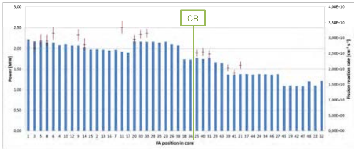
Figure 2.5 - Power/FA and detector response at BoL with all CRs partially inserted in the core. The results are plotted according to the distance from core centre (FA numbering as explained in Figure 2.4).
