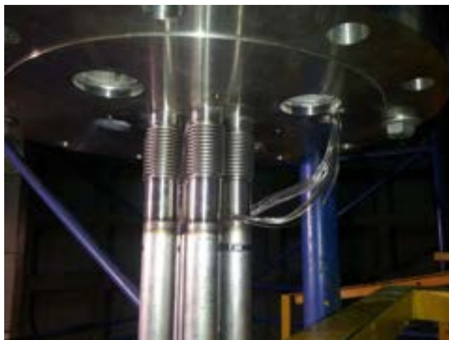
d) HERO test section, thermal compensators
