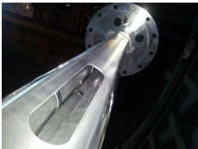
Fig. 14 – HERO-CIRCE SGBT unit: bayonet tubes inserted inside the wrap.
