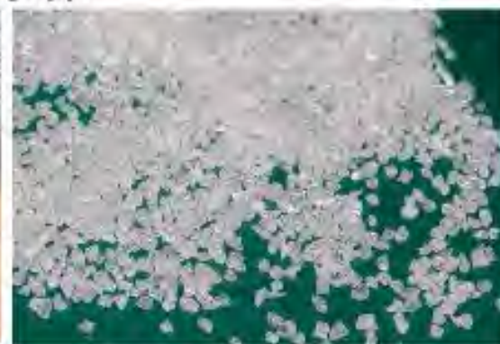
Fused corundum (screened size Al 2 O 3 ) Granular size - 0.8-1.2 mm, Heat resistance >1000°C
