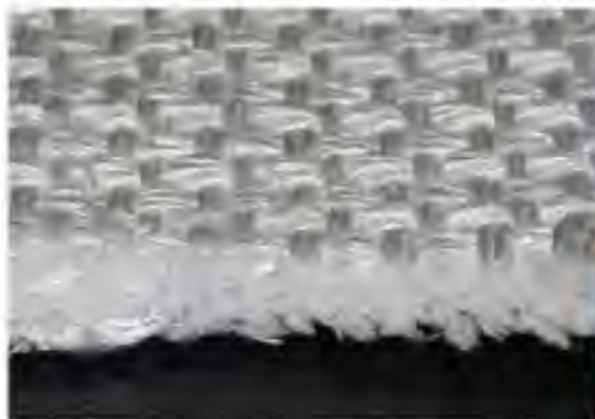
Fiber glass MKTT-2,2A SiO 2 >95 %, Fiber diameter ~ 6μm, Heat resistance - 450°C
