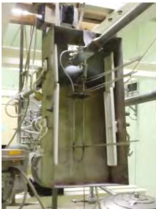
Figure 8 - R-meter installation on the purification branch
