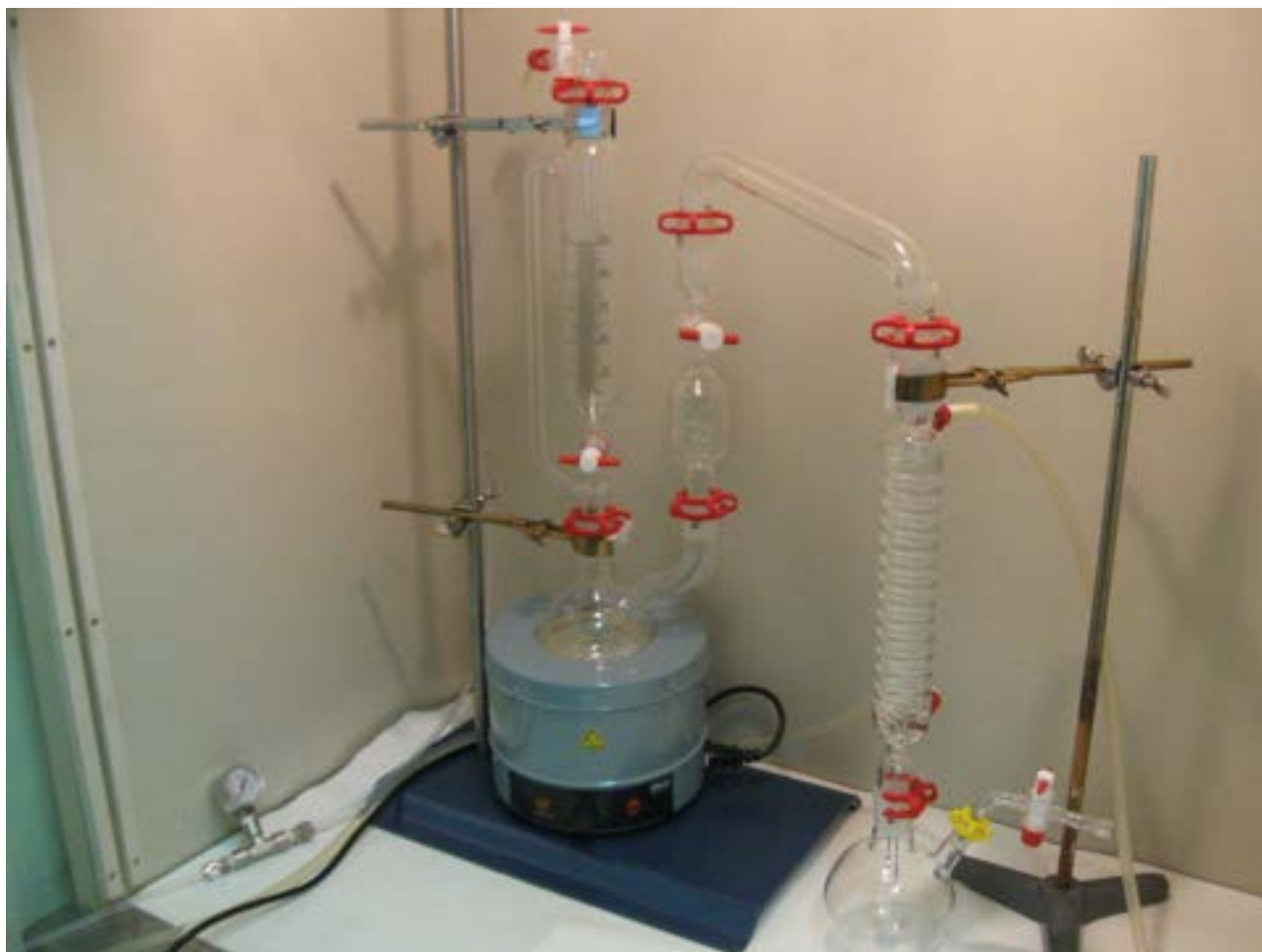
Figure 4: glassware apparatus for the offline chemical analysis of sampled Lithium, inside the chemical hood.
