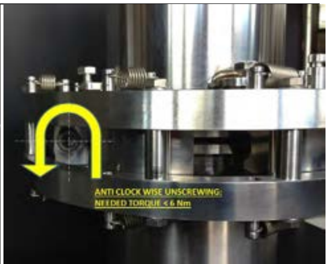
Fig. 12 Emergency opening system
