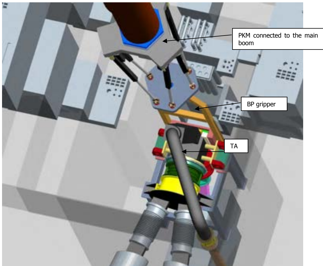
Fig. 2.21 - BP removal in Test Cell
