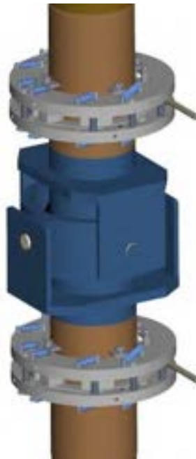
Fig. 2.8 - Detail of the cardan expansion joint
