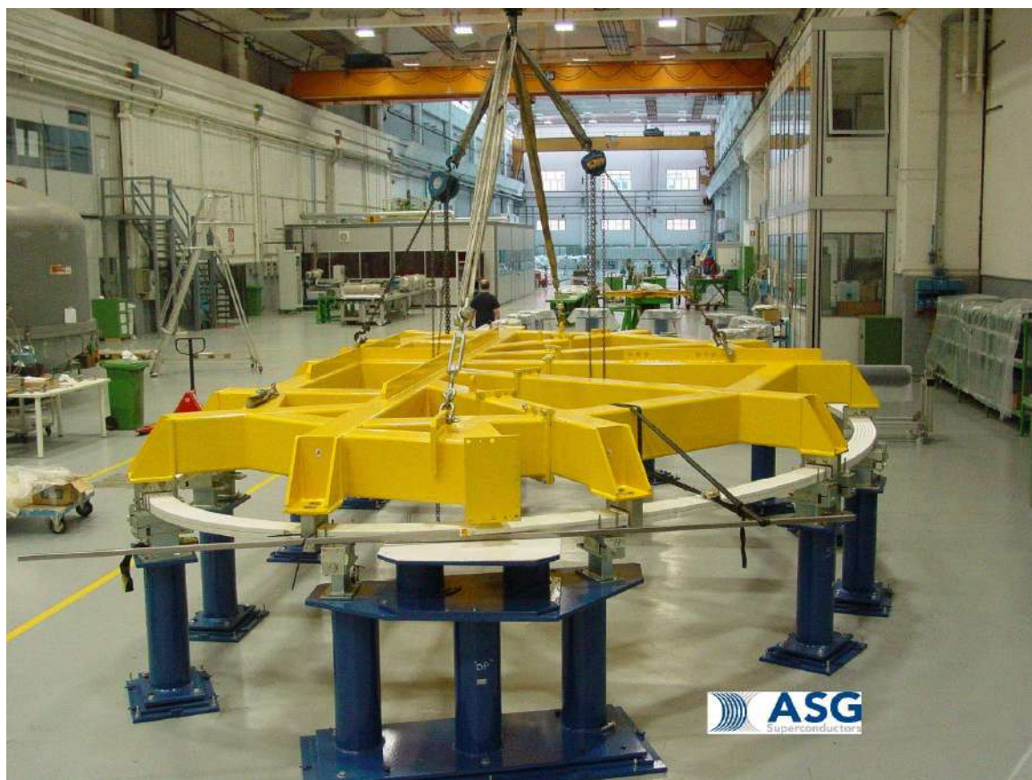
Figure 10 DP positioning on ground insulation bench
