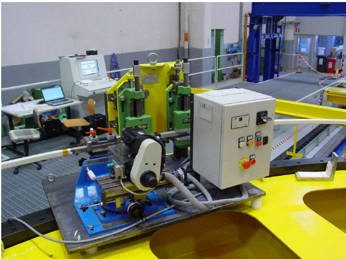
Figure 5 Layer jump and He inlet opening
