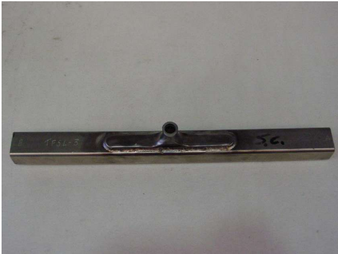
Fig. 1 He inlet insert welded on JT-60SA TF jacket
