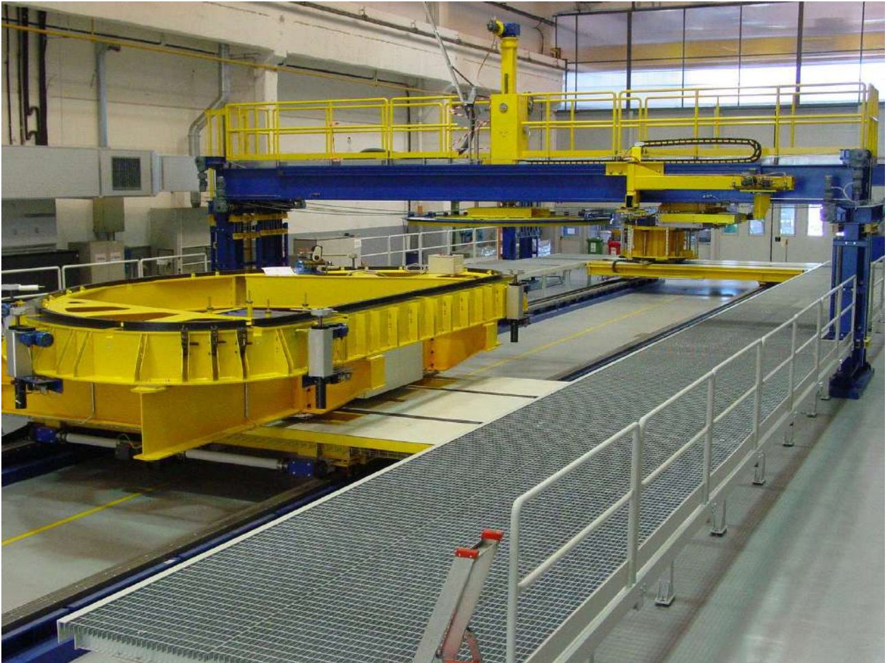
Figure 1 Overview of the winding line for the JT-60SA project in ASG Superconductors in Genoa
