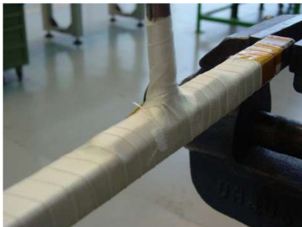
Fig. 12 – Campione He-inlet isolato / He-inlet insulation sample
