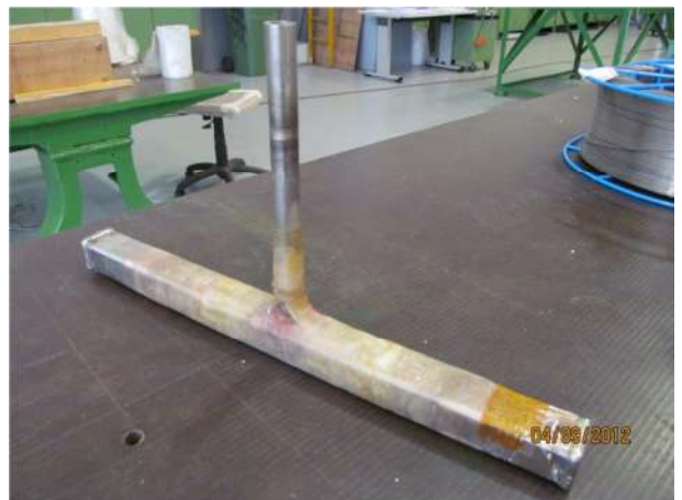
Fig. 12 – Campione He-inlet isolato / He-inlet insulation sample
