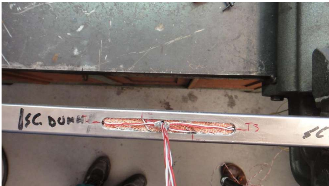
Fig. 2 Welding sample adopted to monitor the temperatures on the cable during welding
