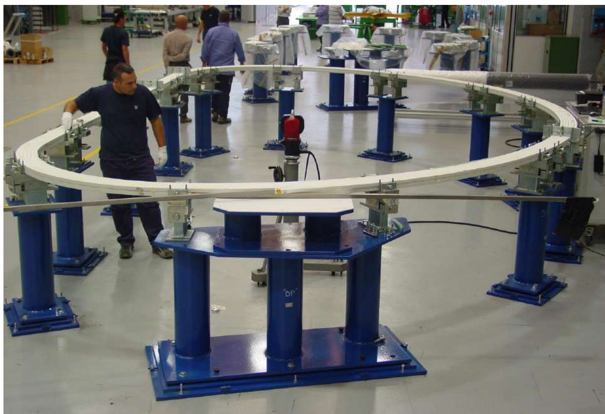
Figure 11 Dimensional survey on DP with laser tracker
