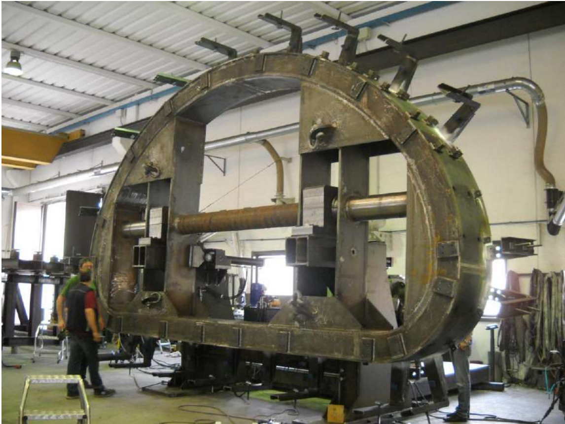
Figure 16 Tooling for WP into casing insertion in vertical position.
