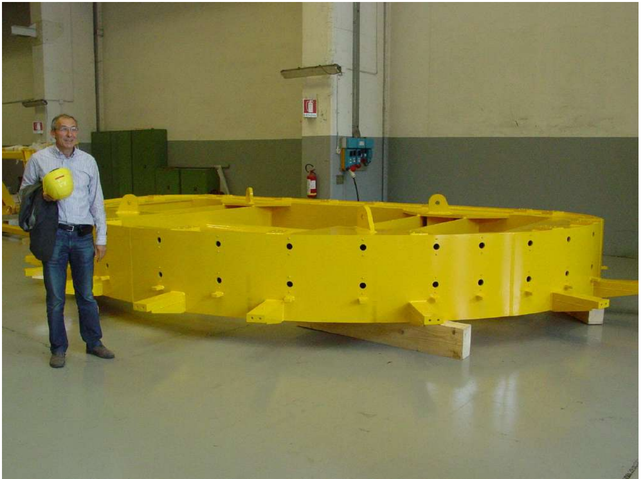
Figure 18 Central core of the WP into casing insertion tooling ready for assembly in ASG workshop.
