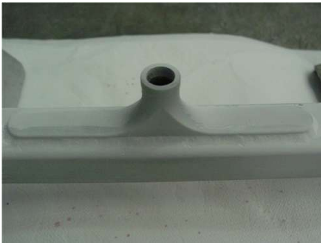
Fig.9.1-9.2 - Test liquidi penetranti / Dye penetrant test
