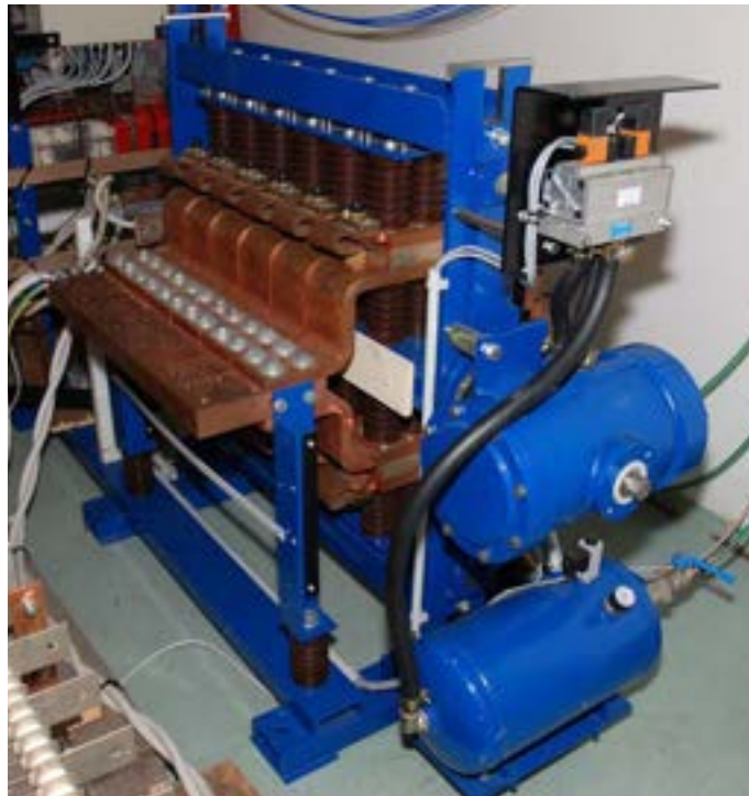
Figure 4.1 – Picture of the BPS used for the Hybrid CB prototype
