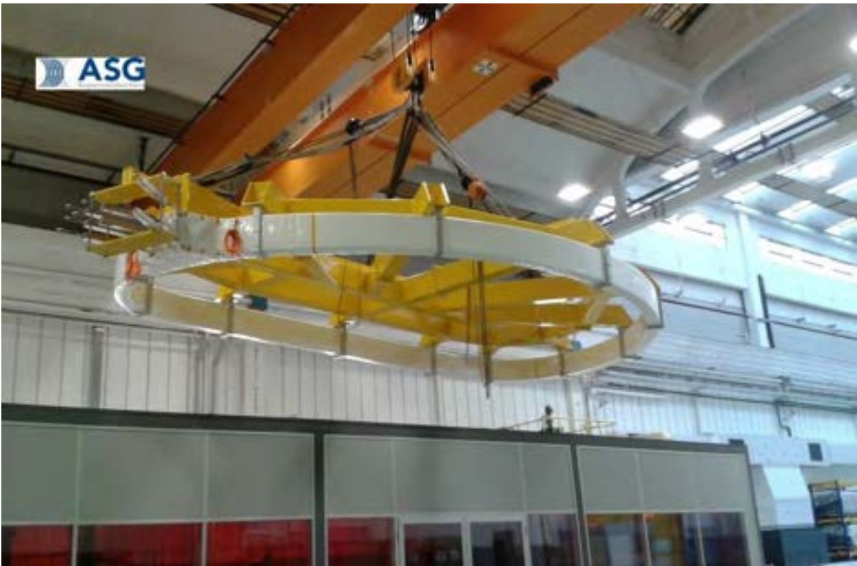
Fig.9 WP01 being transferred to impregnation area
