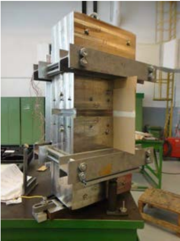
Fig. 24. Curved leg mock-up ready for transverse welding.
