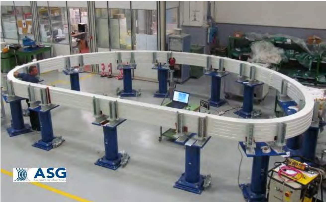
Fig.7 WP01 at the completion of stacking process
