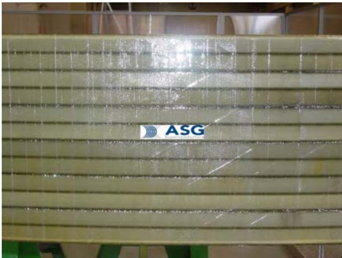
Fig. 13 – Visual inspection of WP01 impregnation
