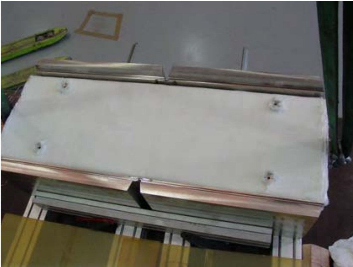
Fig. 20. Curved leg mock-up with beam inserted.
