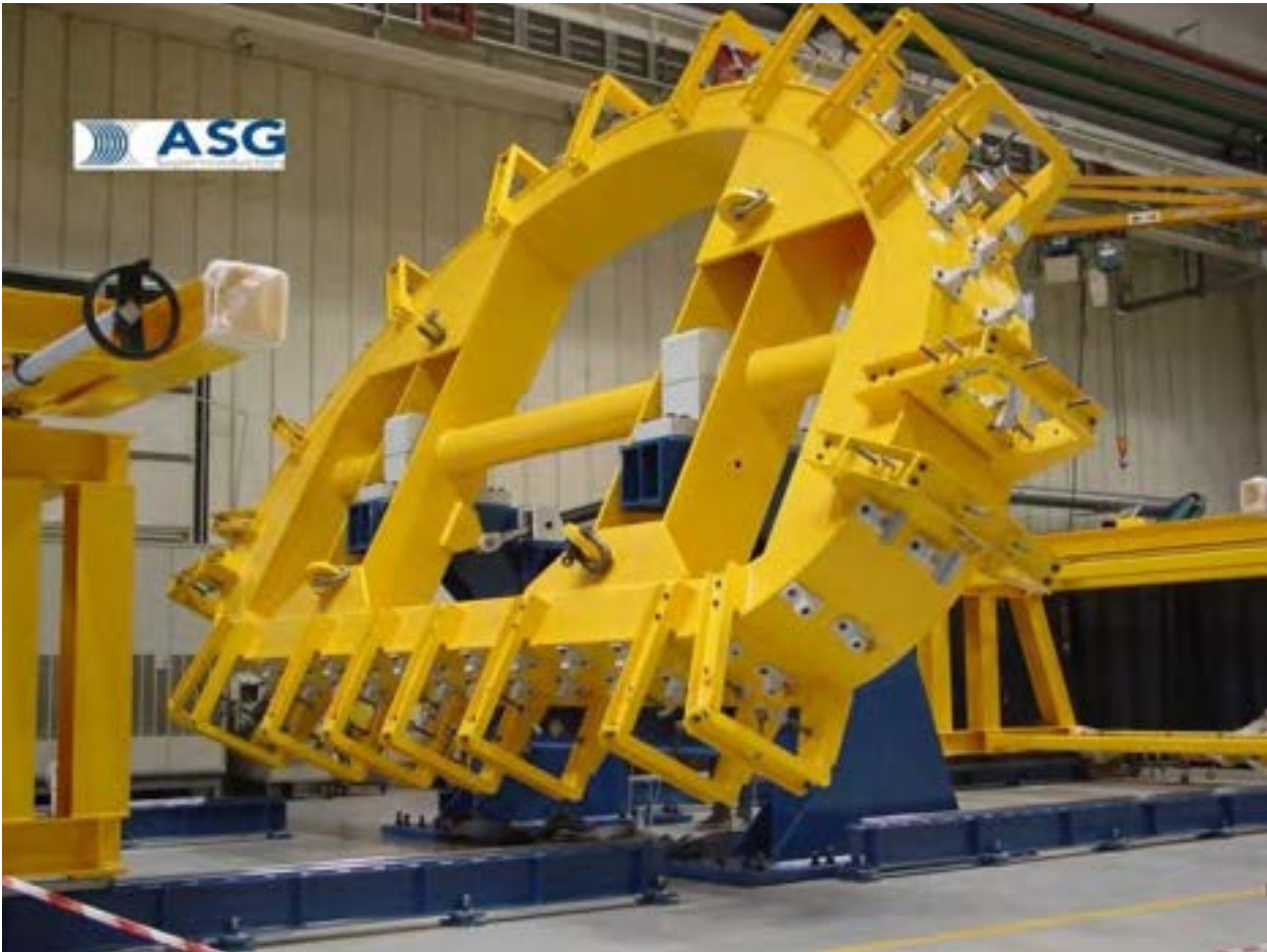
Fig.17 – Tooling for WP insertion into the casing.
