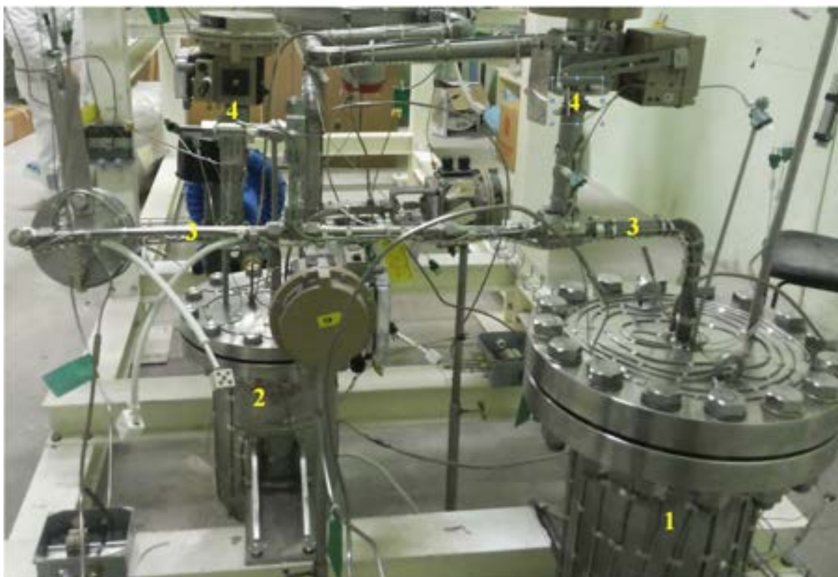
Figure 3: final installation of the Hot Trap inside Lifus 6. 1: Hot Trap; 2: Storage Tank; 3: Pipe connecting the Hot Trap and the Storage Tank; 4: Pneumatic valves
