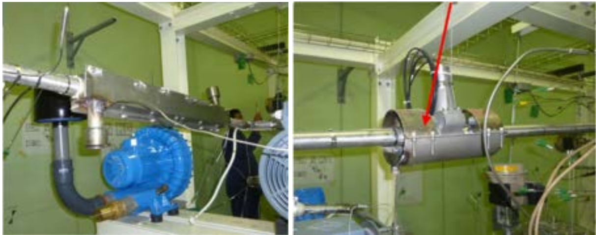
Figure 7: left: main loop Aircooler (3 kW); right: Lithium leak basin
