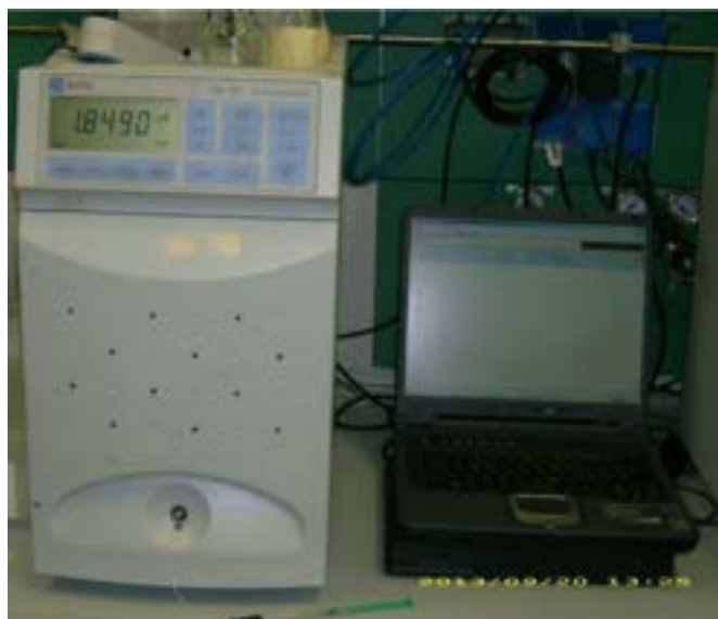
Figure 1: Dionex DX-120 employed by the University of Firenze for the Ammonium Ion ( \text{NH}_4^+ ) analysis, together with the interfaced PC
