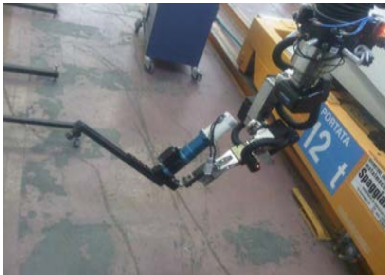
Fig. 12. Light manipulator attached to the TMS
