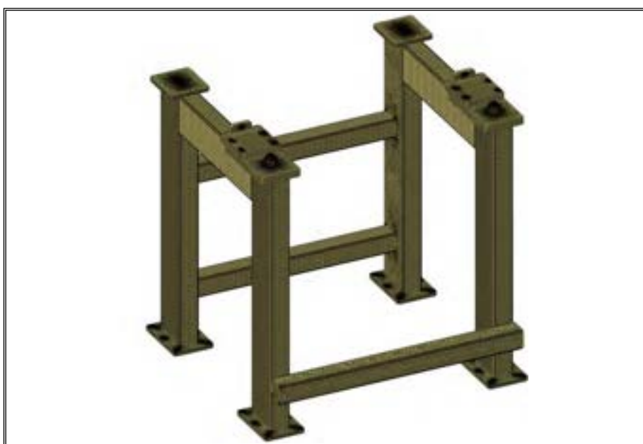
Figure 13. FEM model - Particular of the support framework.
