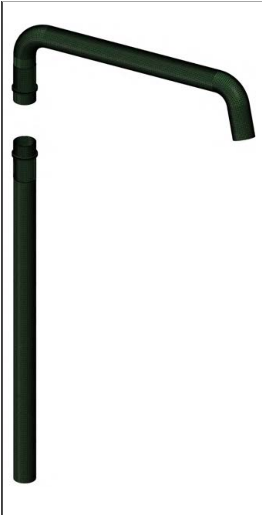
Figure 14. FEM model - Particular of the lithium inlet pipe.
