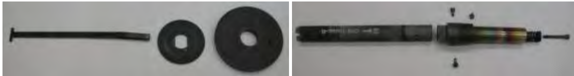
Figure 14: explosion view of the sample holder
