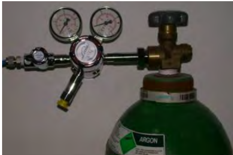
Figure 43: Establish a pressure in the argon line
