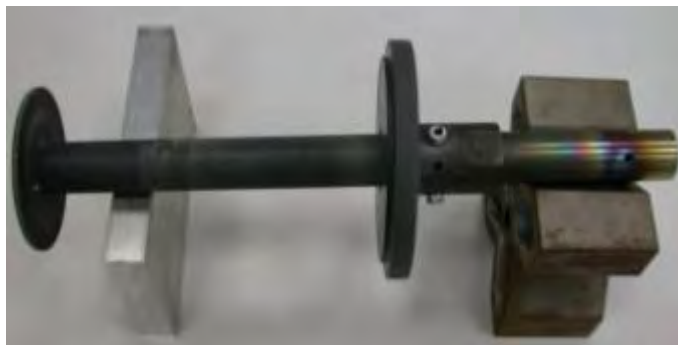
Figure 16: Crucible cup and specimen on the silicon carbide tube
