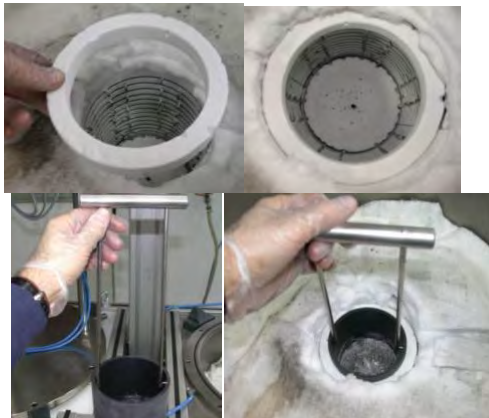
Figure 28: Insertion of the crucible in the furnace
