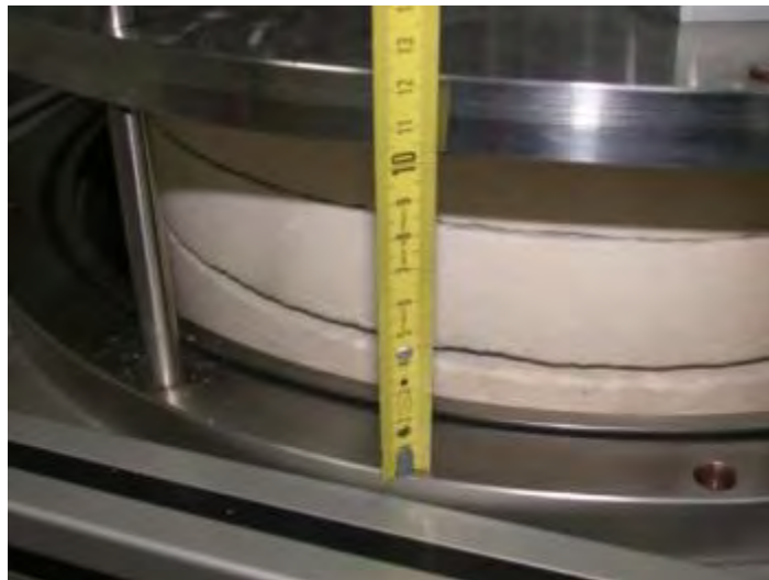
Figure 33: lowering of the closure flange at 100 mm
