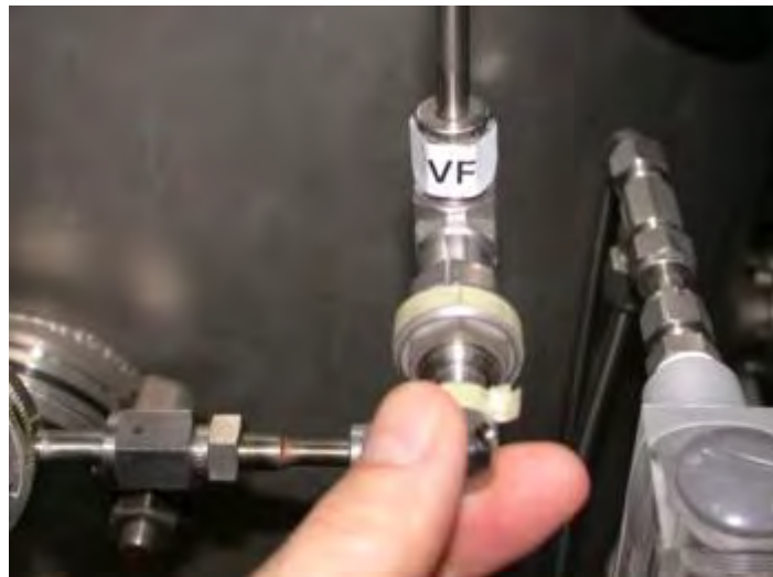
Figure 45: position of the manual regulator valve VF
