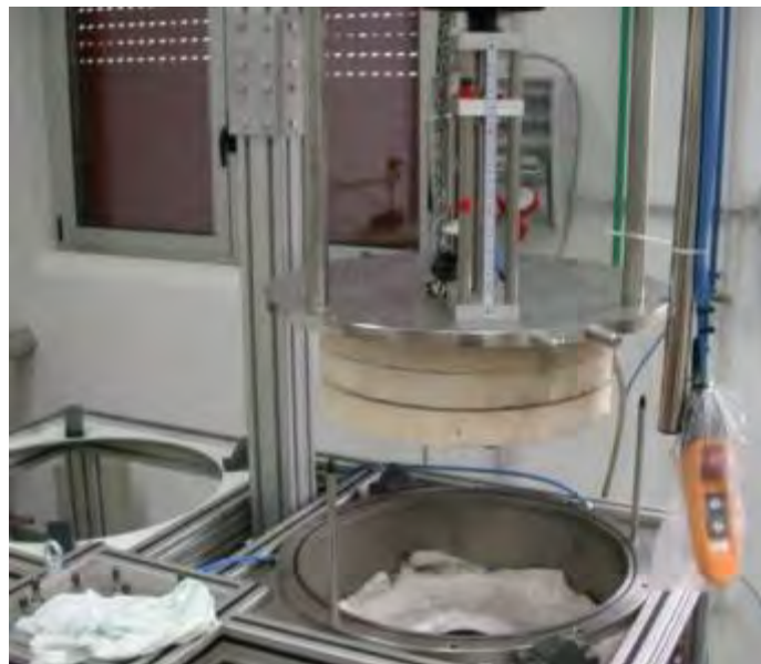
Figure 21: Lifting of the closure flange
