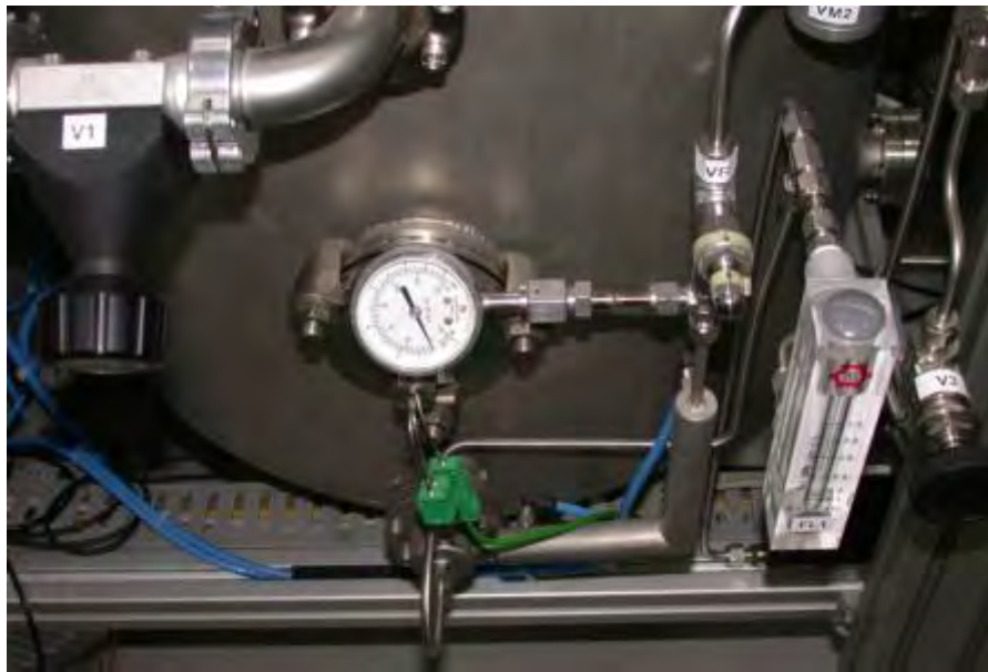
Figure 42a: Position of the argon system valves
