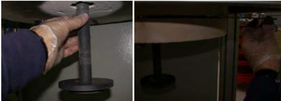
Figure 24: Mount the sample holder on the steel rotating tube
