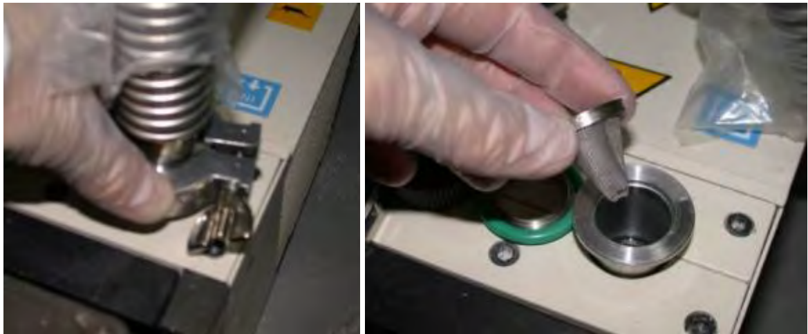
Figure 42: Cleaning of the vacuum pump filter
