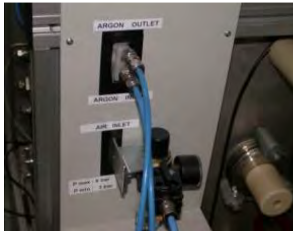
Figure 6: Inlet/outlet argon and inlet air pressure
