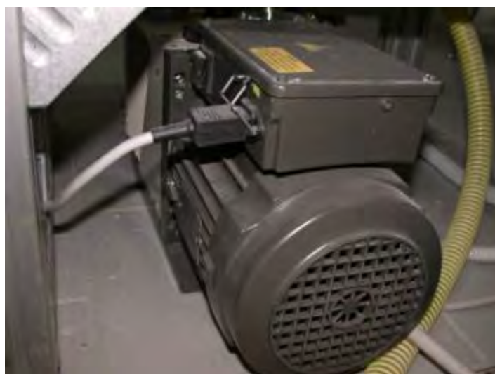
Figure 5: Vacuum pump electrical connections
