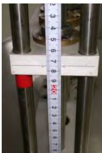
Figure 23: Manual translation system at 175 mm
