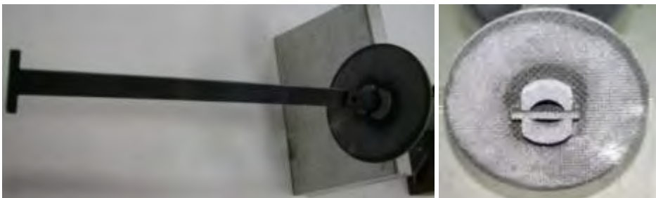
Figure 18: (a) Placing of the tension rod inside the silicon carbide, (b) Placing of the end of the tension rod in the slot of the silicon carbide tube
