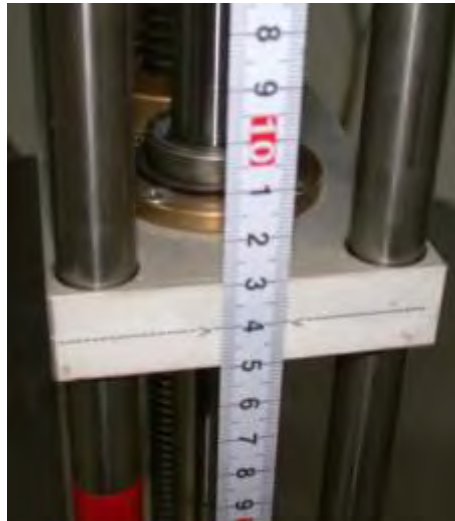
Figure 34: Manual translation system at 140 mm
