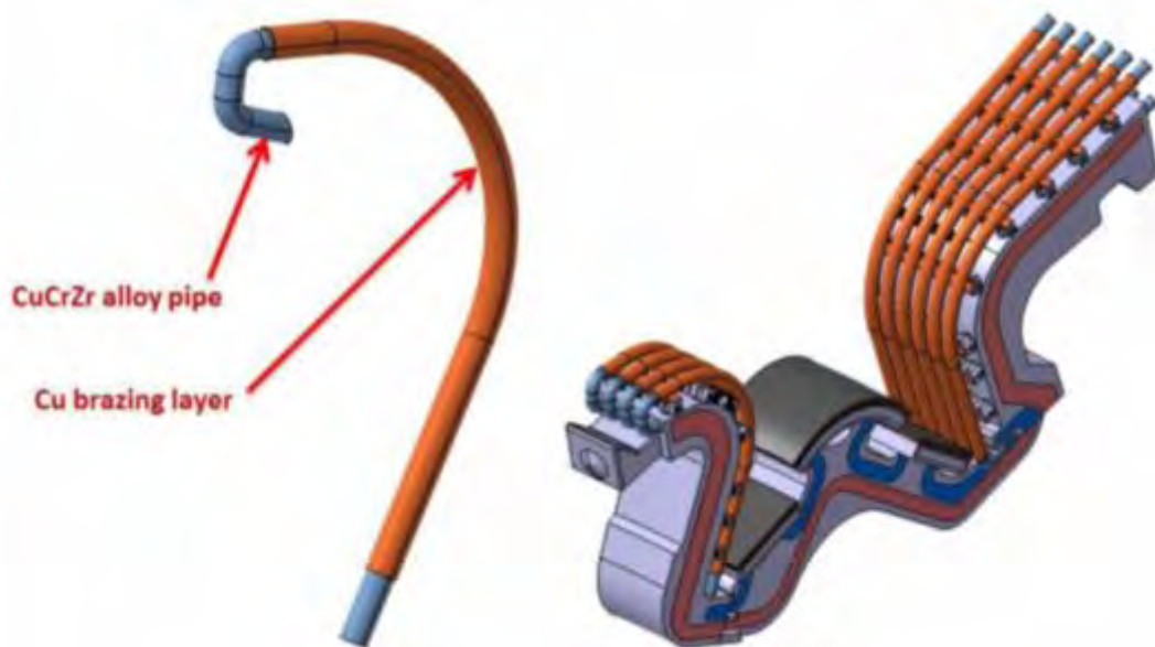
Fig. 22 Divertor New Coolant Layout
