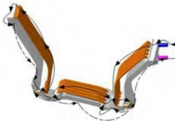
Fig. 27 Cooling channel system of EAST divertor
