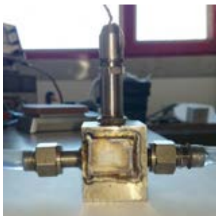
Figure 13: Flowmeter with welded cover sheet
