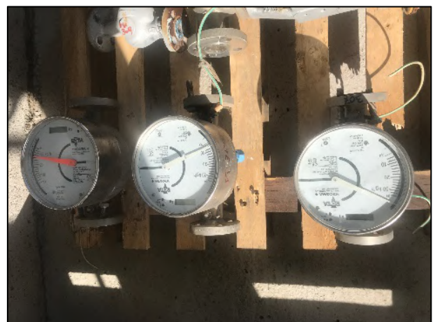
Figura 4.28 – Rotametri FT305, FT306, FT307.
