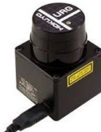
Figura 4 – Sensore laser LRF URG-04LX-UG01 (Hokuyo Automatic Co., Ltd - Japan)
