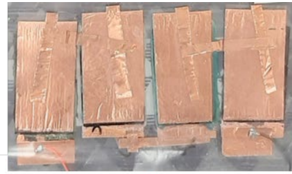
Low-cost, eco-friendly 5V supercapacitor prototype (0.3 F).
