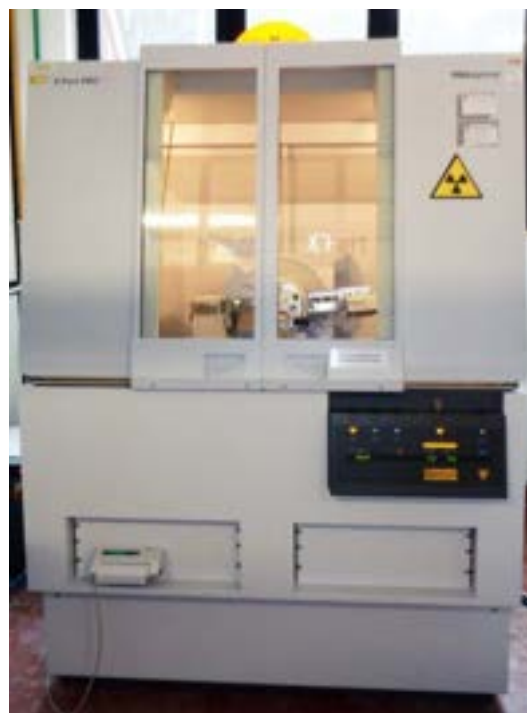
Figura 16. Diffrattometro PANalytical X'Pert PRO
