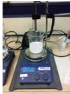
10.2. Mixing nitrato Al e CaO 70°C; 1 h
