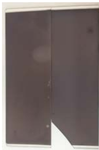
KN640: niente S – uscita chiusa! T_{\text{forno}}=585 , T_{\text{piattello}}=545 , t_{\text{dwell}}=30' \Phi_{\text{carrier}}=0 ; \Phi_{\text{N}_2}=0 T_{\text{S}_2}=30^\circ\text{C} – senza crogiuolo
