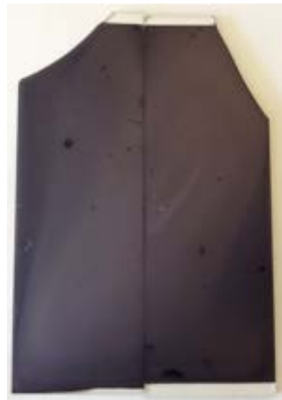
KN645: base poli c-Si + zolfo T_{\text{forno}}=585 , T_{\text{piattello}}=545 , t_{\text{dwell}}=30' \Phi_{\text{carrier}}=1 l/min ; \Phi_{\text{N}_2}=0 T_{\text{S}_2}=190^\circ\text{C} + con crogiuolo - SP499-SP250
