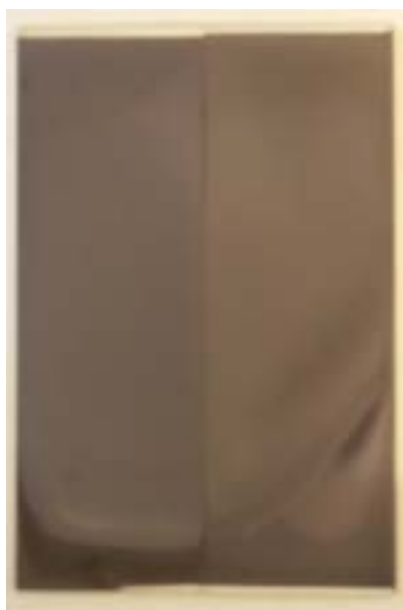
KN642: niente S T_{\text{forno}}=585 , T_{\text{piattello}}=545 , t_{\text{dwell}}=30' \Phi_{\text{carrier}}=1 l/min; \Phi_{\text{N}_2}=0 T_{\text{S}_2}=190^\circ\text{C} – senza crogiuolo
