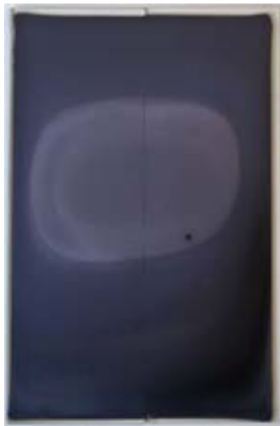
KN634: cornice grafite T_{\text{piattello}}=545 , T_{\text{forno}}=585 t_{\text{dwell}}=60' \Phi_{\text{carrier}}=1 l/min; \Phi_{\text{N}_2}=0.5 l/min T_{\text{S}_2}=190^\circ\text{C} (Sp241)
