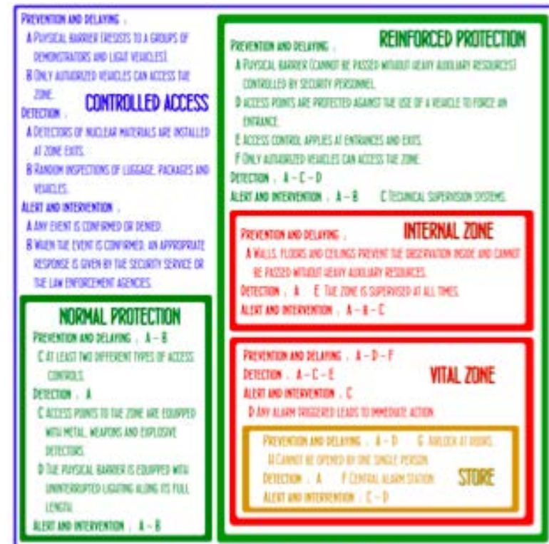
Fig. 4.3: Physical Protection System in France.
