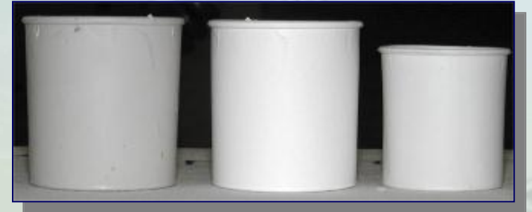
Campioni stampati in \text{Al}_2\text{O}_3
